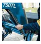
SECURE AND EASY TO CHECK Protected within the under boom channel section, the hydraulic lines remain easy to inspect.
